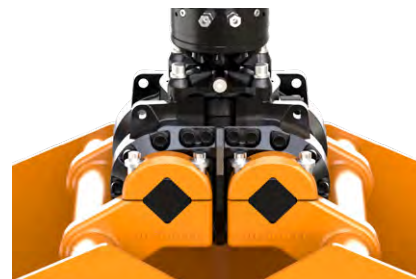
Loosen 4 bolts on each side
